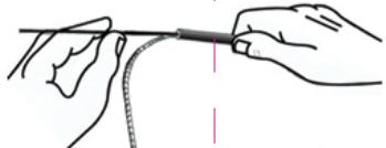
7. If the repair involves replacing ferrules, use waterproof glue to secure
