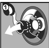
To begin inflation open external cap and pull firmly on lanyard to extend out. This will open internal seal.
