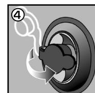
Fully remove pump and close external stopper. Valve should appear depressed into itself.
